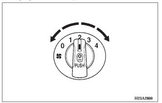
The blower may be operated (when the ignition key is in the ON position) at 4 different speeds. Select the best speed to fit your needs. When the blower switch is set to the "O" position, all air conditioning functions will stop.
